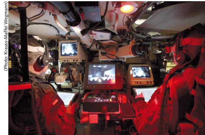
The central control unit and the MDU display as a user interface in the Puma
